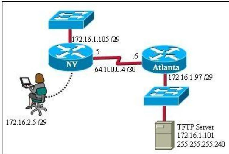
A TFTP server has recently been installed in the Atlanta office. The network administrator is located in the NY office and has made a console connection to the NY router. After establishing the connection they are unable to backup the configuration file and IOS of the NY router to the TFTP server. What is the cause of this problem?
