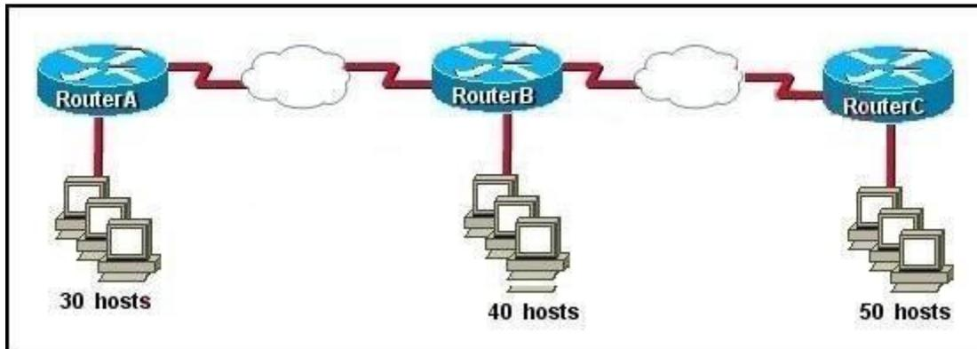
The enterprise has decided to use the network address 172.16.0.0. The network administrator needs to design a classful addressing scheme to accommodate the three subnets, with 30, 40, and 50 hosts, as shown. What subnet mask would accommodate this network?
