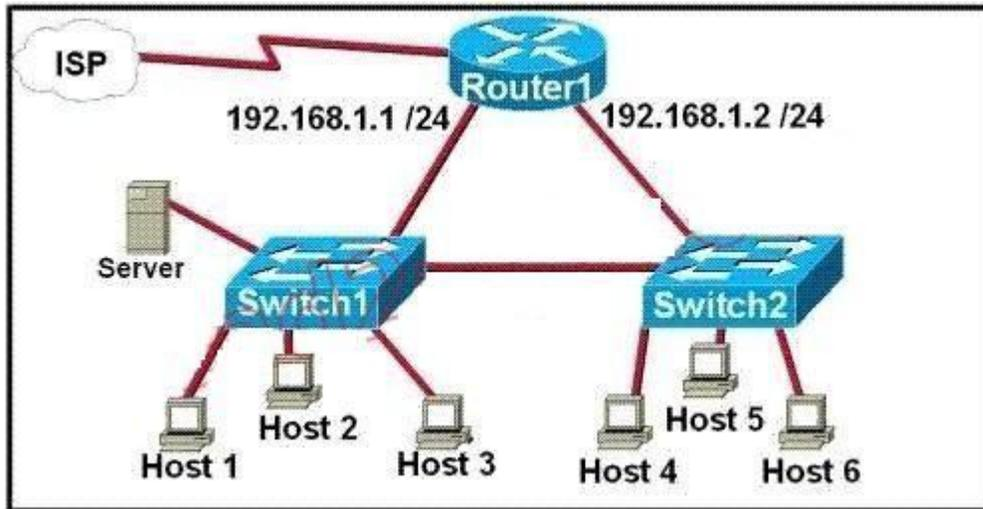
A network technician is asked to design a small network with redundancy. The exhibit represents this design, with all hosts configured in the same VLAN. What conclusions can be made about this design?
