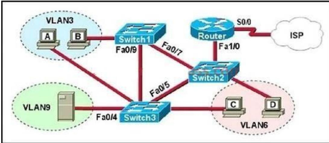
A problem with network connectivity has been observed. It is suspected that the cable connected to switch port Fa0/9 on Switch1 is disconnected. What would be an effect of this cable being disconnected?
