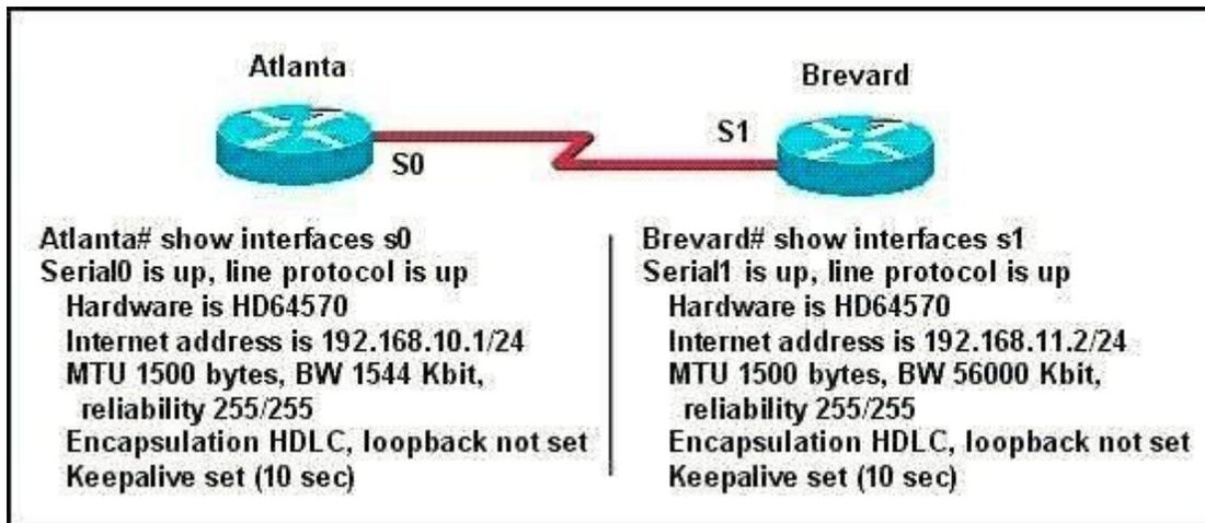
Given the partial configurations shown in the exhibit, what is the problem on the Brevard router that is causing the lack of connectivity?
