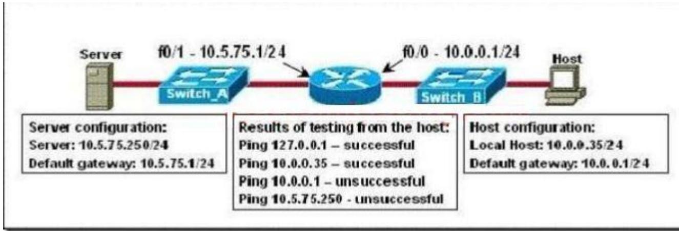
A technician is troubleshooting a host connectivity problem. The host is unable to ping a server connected to Switch\_A. Based on the results of the testing, what could be the problem?
