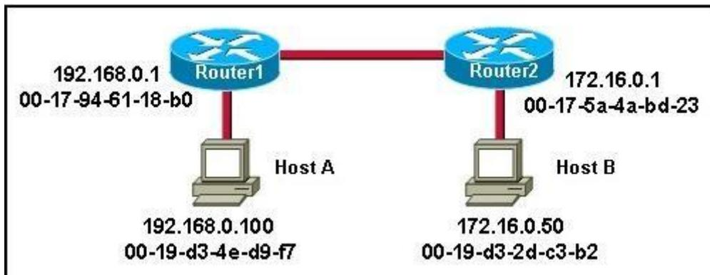
Host A is sending a packet to Host B for the first time. What destination MAC address will Host A use in the ARP request?
