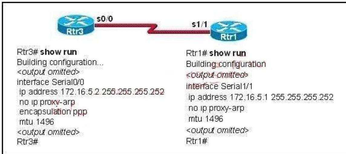
A network administrator is troubleshooting a connectivity problem on the serial interfaces. The output from the show interfaces command on both routers shows that the serial interface is up, line protocol is down. Given the partial output for the show running-config in the exhibit, what is the most likely cause of this problem?
