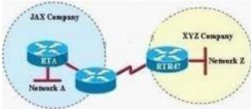
A person is trying to send a file from a host on Network A of the JAX Company to a server on Network Z of the XYZ Company. The file transfer fails. The host on Network A can communicate with other hosts on Network A.
