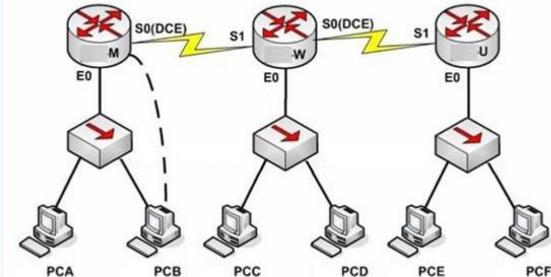
**Note.** The OSPF process must be configured to allow interfaces in specific subnets to participate in the routing process.
