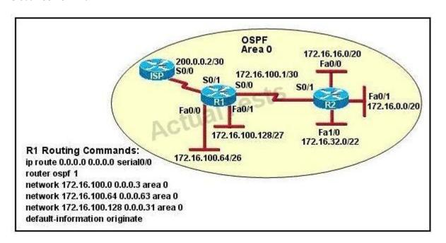
Assume that all router interfaces are operational and correctly configured. In addition, assume that OSPF has been correctly configured on router R2. How will the default route configured on R1 affect the operation of R2?
