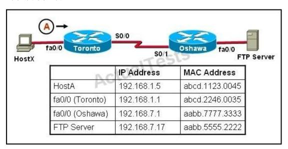
HostX is transferring a file to the FTP server. Point A represents the frame as it goes toward the Toronto router. What will the Layer 2 destination address be at this point?
