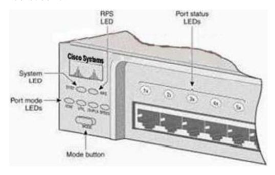
After the power-on-self test (POST), the system LED of a Cisco 2950 switch turns amber. What is the status of the switch?
