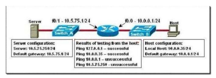
A technician is troubleshooting a host connectivity problem. The host is unable to ping a server connected to Switch\_A. Based on the results of the testing, what could be the problem?
