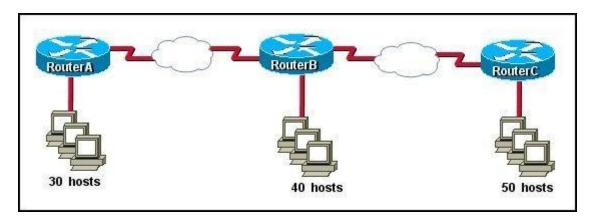
The internetwork is using subnets of the address 192.168.1.0 with a subnet mask of 255.255.255.224. The routing protocol in use is RIP version 1. Which address could be assigned to the FastEthernet interface on RouterA?
