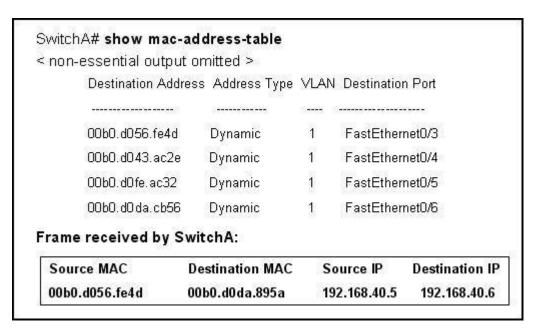
SwitchA receives the frame with the addressing shown in the exhibit. According to the command output also shown in the exhibit, how will SwitchA handle this frame?
