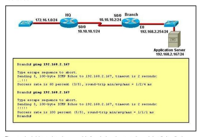
The network administrator is testing connectivity from the branch router to the newly installed application server. What is the most likely reason for the first ping having a success rate of only 60 percent?
