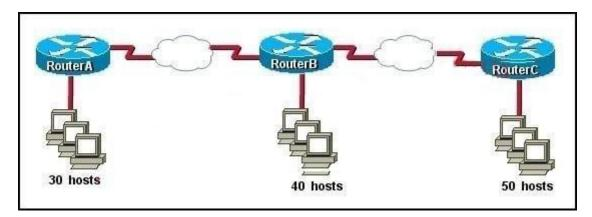
The enterprise has decided to use the network address 172.16.0.0. The network administrator needs to design a classful addressing scheme to accommodate the three subnets, with 30, 40, and 50 hosts, as shown. What subnet mask would accommodate this network?
