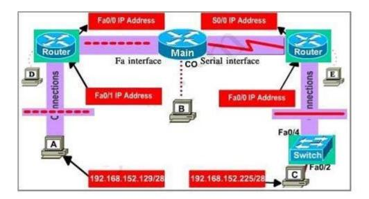
Assign appropriate IP addresses for interfaces:
