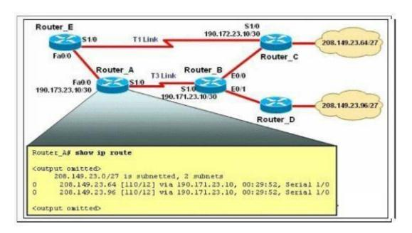
The network is converged. After link-state advertisements are received from Router\_A, what information will Router\_E contain in its routing table for the subnets 208.149.23.64 and 208.149.23.96?
