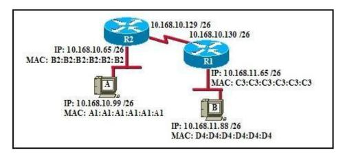
If host A sends an IP packet to host B, what will the source physical address be in the frame when it reaches host B?
