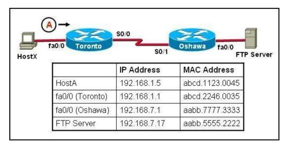
HostX is transferring a file to the FTP server. Point A represents the frame as it goes toward the Toronto router. What will the Layer 2 destination address be at this point?
