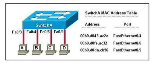
The exhibit is showing the topology and the MAC address table. Host A sends a data frame to host D. What will the switch do when it receives the frame from host A?
