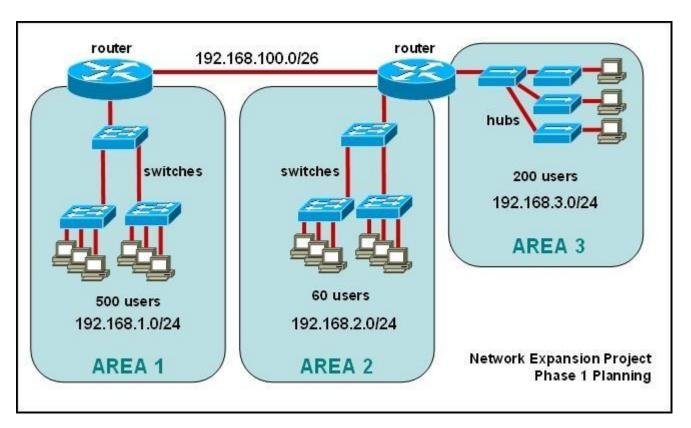
The junior network support staff provided the diagram as a recommended configuration for the first phase of a four-phase network expansion project. The entire network expansion will have over 1000 users on 14 network segments and has been allocated this IP address space.
