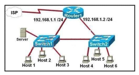
A network technician is asked to design a small network with redundancy. The exhibit represents this design, with all hosts configured in the same VLAN. What conclusions can be made about this design?
