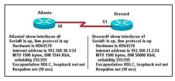
Given the partial configurations shown in the exhibit, what is the problem on the Brevard router that is causing the lack of connectivity?
