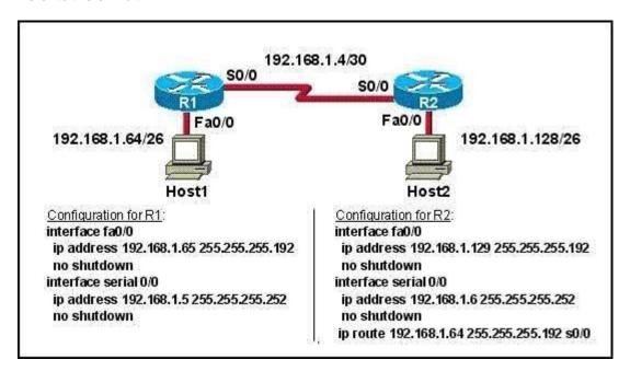
A technician pastes the configurations in the exhibit into the two new routers shown. Otherwise, the routers are configured with their default configurations. A ping from Host1 to Host 2 fails, but the technician is able to ping the S0/0 interface of R2 from Host 1. The configurations of the hosts have been verified as correct. What could be the cause of the problem?
