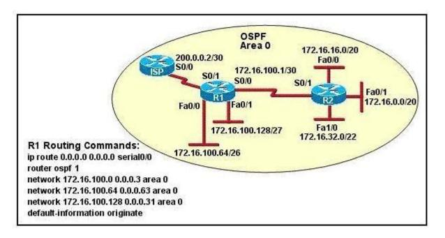
Assume that all router interfaces are operational and correctly configured. In addition, assume that OSPF has been correctly configured on router R2. How will the default route configured on R1 affect the operation of R2?
