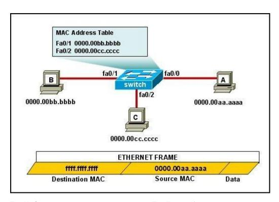
The MAC address table is shown in its entirety. The Ethernet frame that is shown arrives at the switch. What two operations will the switch perform when it receives this frame? (Choose two.)
