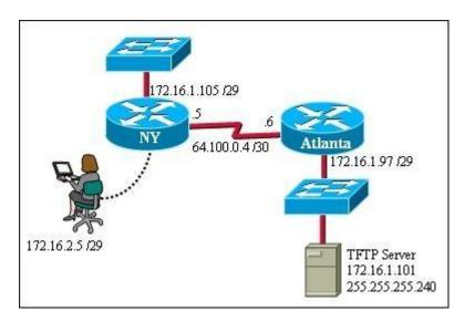
A TFTP server has recently been installed in the Atlanta office. The network administrator is located in the NY office and has made a console connection to the NY router. After establishing the connection they are unable to backup the configuration file and IOS of the NY router to the TFTP server. What is the cause of this problem?
