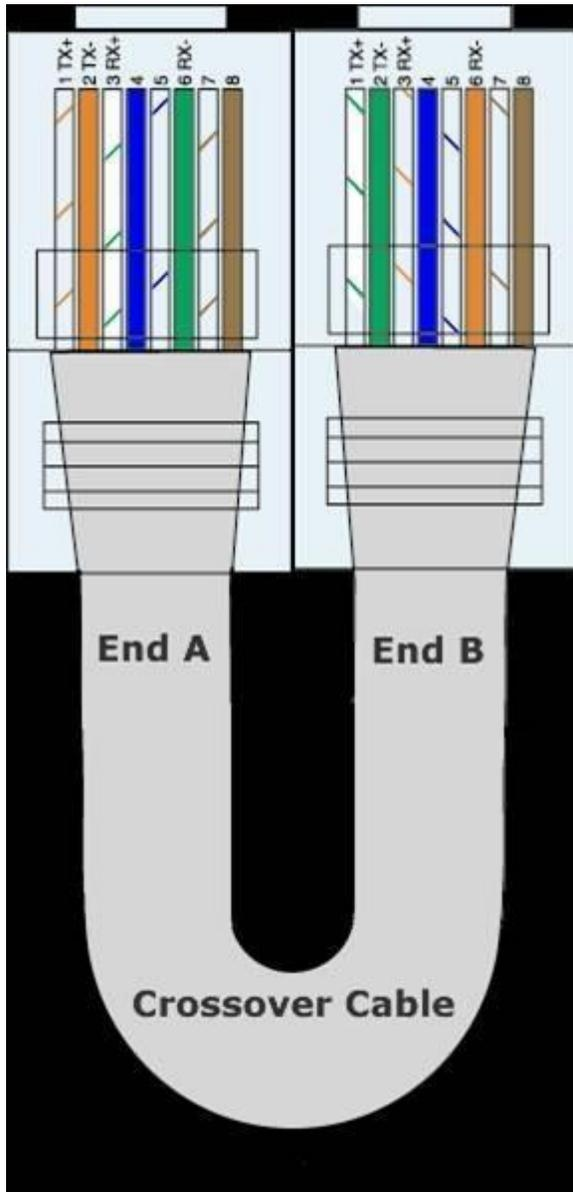
The wire scheme that is shown is terminated at each end with an RJ-45 connector. What cable type does the wire diagram represent?
