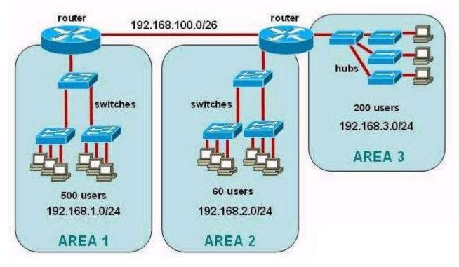
A The AREA 1 IP address space is inadequate for the number of users. B The AREA 3 IP address space is inadequate for the number of users. C - AREA 2 could use a mask of /25 to conserve IP address space. D The network address space that is provided requires a single network-wide mask. E The router-to-router connection is wasting address space. F The broadcast domain in AREA 1 is too large for IP to function.
