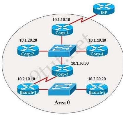
The internetwork infrastructure of company XYZ consists of a single OSPF area as shown in the graphic. There is concern that a lack of router resources is impeding internetwork performance.
