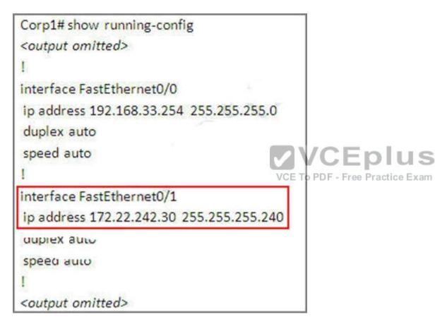
We learn that interface FastEthernet0/1 is the interface connected to Server LAN network. It is the interface we will apply our access-list (for outbound direction). **Corp1#configure terminal**
