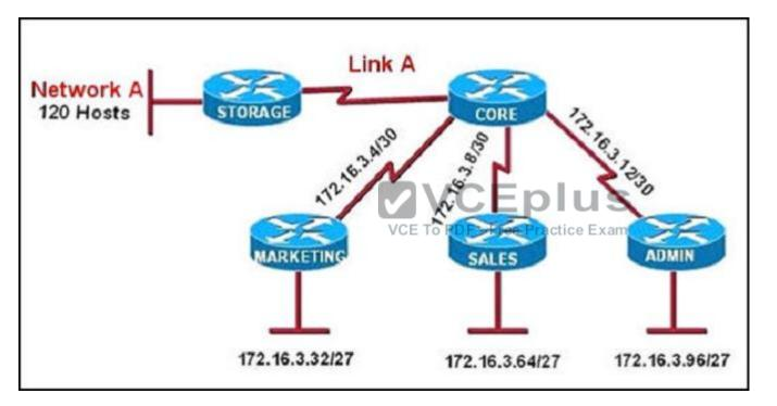
All of the routers in the network are configured with the ip subnet-zero command. Which network addresses should be used for Link A and Network A? (Choose two.)
