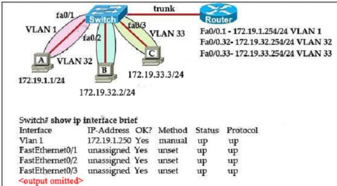
The network administrator normally establishes a Telnet session with the switch from host A. However, host A is unavailable. The administrator's attempt to telnet to the switch from host B fails, but pings to the other two hosts are successful. What is the issue?
