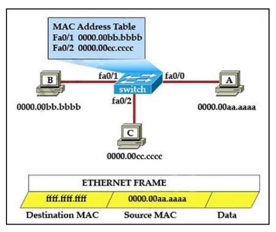
The MAC address table is shown in its entirety. The Ethernet frame that is shown arrives at the switch. What two operations will the switch perform when it receives this frame? (Choose two.)
