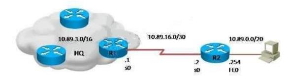
Which command is simplest to configure routing between the regional office network 10.89.0.0/20 and the corporate network?
