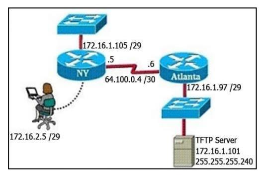
A TFTP server has recently been instated in the Atlanta office. The network administrator is located in the NY office and has made a console connection to the NY router. After establishing the connection they are unable to backup the configuration file and iOS of the NY router to the TFTP server. What is the cause of this problem?
