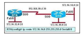
RTA is configured with a basic configuration. The link between the two routers is operational and no routing protocols are configured on either router. The line shown in the exhibit is then added to router RTA. Should interface Fa0/0 on router RTB shut down, what effect will the shutdown have on router RTA?
