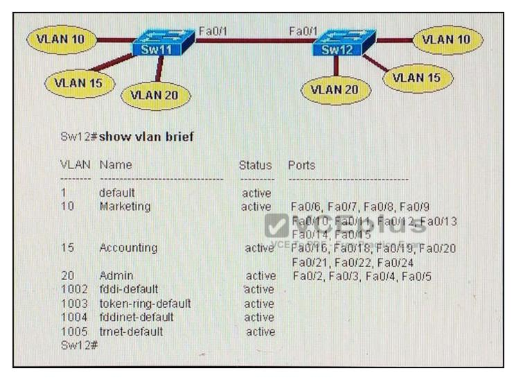
Refer to the exhibit. A technician has configured the FastEthernet0/1 interface on Sw11 as an access link in VLAN 1. Based on the output from the **show vlan brief** command issued on Sw12, what will be the result of making this change on Sw11?
