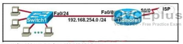
access-list 106 permit ip host 192.168.254.7 any access-list 106 deny icmp 192.168.254.0 0.0.0.255 any echo access-list 106 permit ip any any interface Fa0/0 ip access-group 106 in
