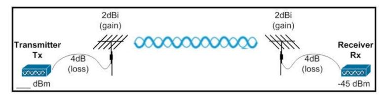
A network engineer needs the far end of a wireless bridge to receive at -45dBM. Based on the diagram, what value in dBm must the transmitter use to send to achieve the desired result?
