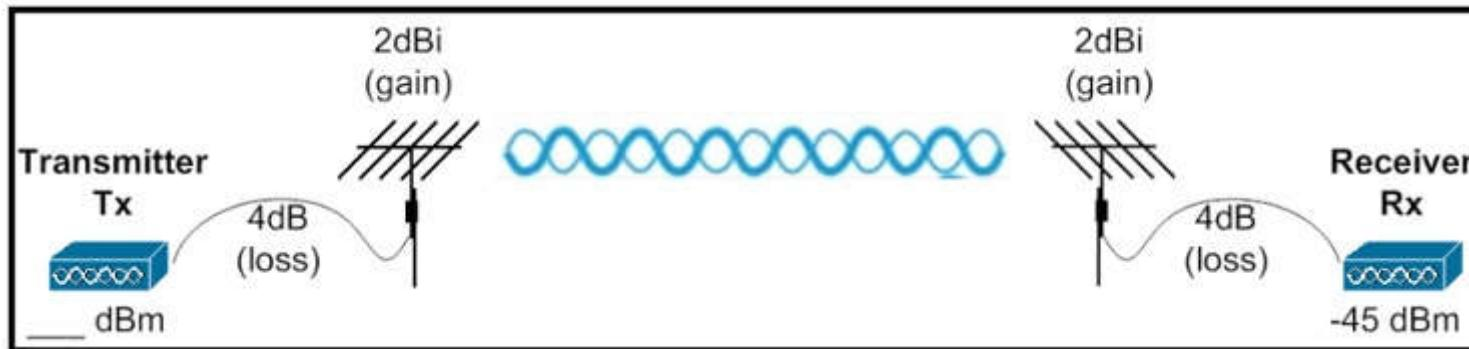
A network engineer needs the far end of a wireless bridge to receive at -45dBm. Based on the diagram, what value in dBm must the transmitter use to send to achieve the desired result?
