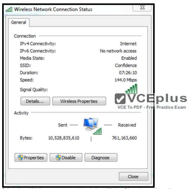
Refer to the exhibit. A customer is determining whether a Windows 7 laptop is operating on the correct IEEE 802.11 standard. Which standard is being used by the laptop in the exhibit?
