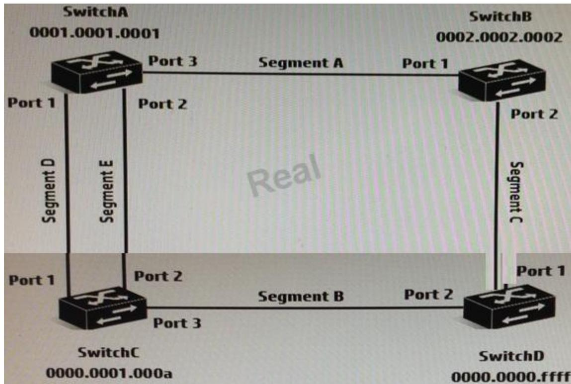
A company has implemented a switched network based on the RSTP spanning tree protocol.
