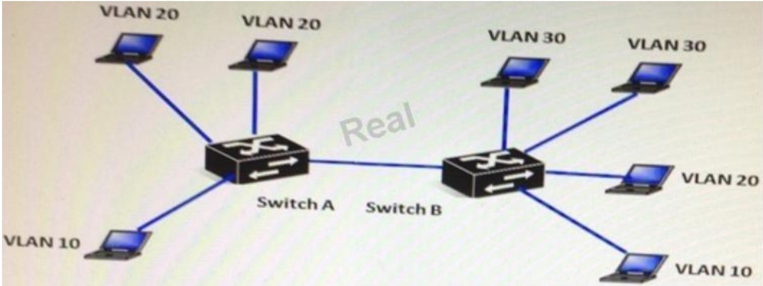
The network consists of two IP ProVision Switches with routing disabled. How should the network administrator configure the link between Switch A and Switch B to ensure all hosts can communicate to all the other hosts within their respective VLANs?
