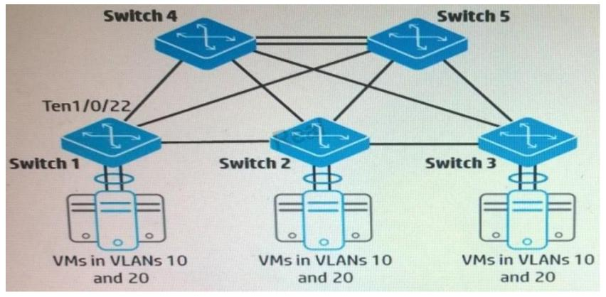
The switch shown in the exhibit should from a TRILL region. For Switch 1 interface ten1/0/22, what is a valid port link-type and TRILL port type?
