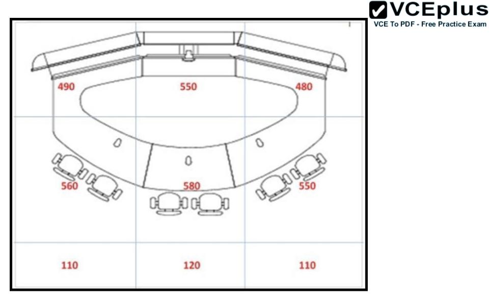
The numbers on the floor plan represent the horizontal average lux readings for nine different room areas. Considering Cisco best practices, what can you conclude about the lighting conditions?
