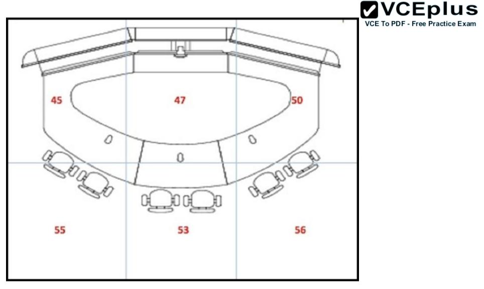
Acoustic measurements for ambient noise were taken on a candidate for an Immersive Cisco TelePresence room. The numbers on the floor plan represent the dBA readings for each of the six areas of the room.
