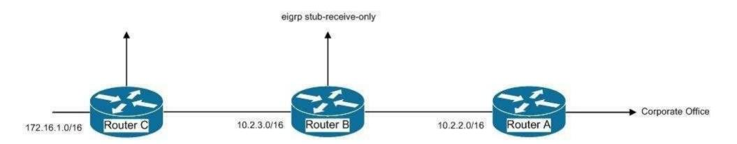
Router A is not receiving the route to the 172.16.1.0/16 network because Router B, which stands between Router A and C, is configured with the eigrp stubreceiveonly command. This is resulting in hosts from the corporate office being unable to connect to hosts in the 172.16.0.0/16 network. If there were a legitimate reason to keep Router B configured with the eigrp stub-receive-only command, the problem could be solved by executing the following command set on Router A:
