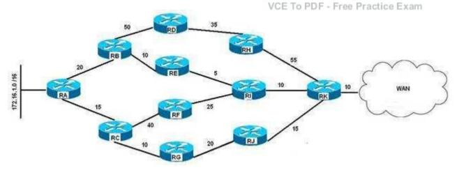
You have configured EIGRP with the variance parameter set to 3 on all the routers to enable unequal load balancing from the 172.16.1.0 network to the WAN. The delay configured on each of the routers is shown in the LAN diagram, and the K values are set as follows:
