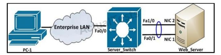
Users of PC-1 experience slow connection when a webpage is requested from the server. To increase bandwidth, the network engineer configured an EtherChannel on interfaces Fa1/0 and Fa0/1 of the server farm switch, as shown here:
