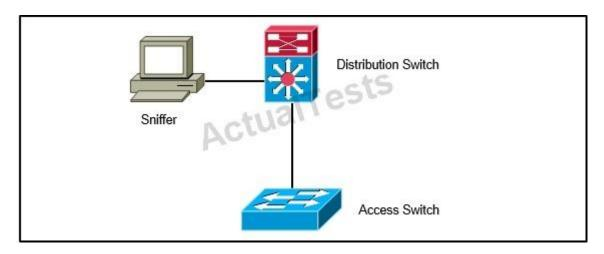
A network engineer wants to analyze all incoming and outgoing packets for an interface that is connected to an access switch. Which three items must be configured to mirror traffic to a packet sniffer that is connected to the distribution switch? (Choose three.)
