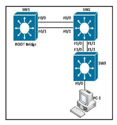
f1/0 and f1/1 have the same end-to-end path cost to the designated bridge. Which action is needed to modify the Layer 2 spanning-tree network so that traffic for PC1 VLAN from switch SW3 uses switchport f1/1 as a primary port?
