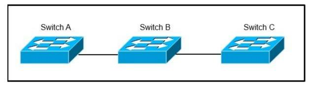
Switch A, B, and C are trunked together and have been properly configured for VTP. Switch C receives VLAN information from the VTP server Switch A, but Switch B does not receive any VLAN information. What is the most probable cause of this behavior?
