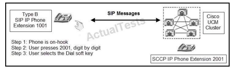
A user is going through a series of dialing steps on a SIP Type B IP phone to call a SCCP IP phone. Both phones are registered to the same Cisco Unified Communications Manager cluster. Assume that the calling SIP phone is associated with a SIP dial rule with a pattern value of "2001".
