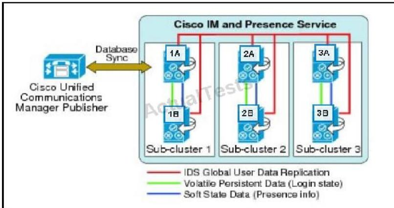
In this high-availability Cisco IM and Presence deployment with three subclusters, the first user is assigned to server 1A; the second user is assigned to server 2A; and the third user is assigned to server 3A. Assume that the Cisco IM and Presence is set to Active/Standby mode, to which server should the fourth user be assigned?
