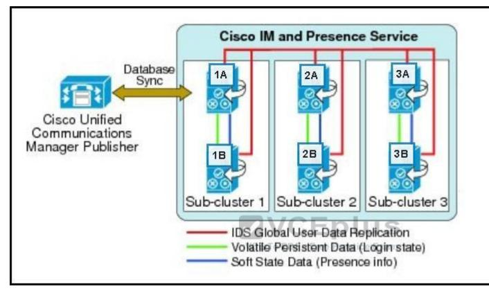
In this high-availability Cisco IM and Presence deployment with three subclusters, the first user is assigned to server 1A; the second user is assigned to server 2A; and the third user is assigned to server 3A. Assume that the Cisco IM and Presence is set to Active/Standby mode, to which server should the fourth user be assigned?
