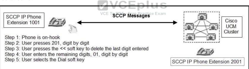
A user is performing a series of dialing steps on a SCCP IP phone (extension 1001) to call another SCCP IP phone (extension 2003). Both phones are registered to the same Cisco Unified Communications Manager cluster.
