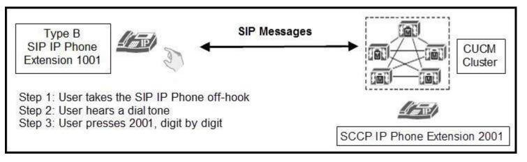
A user is going through a series of dialing steps on a SIP Type B IP phone (for example, a Cisco 7975) to call an SCCP IP phone. Both phones are registered to the same Cisco Unified Communications Manager cluster. Assuming that the calling SIP phone is not associated with any SIP dial rules, which statement about how digits are forwarded to Cisco Unified Communications Manager for further call processing is true?
