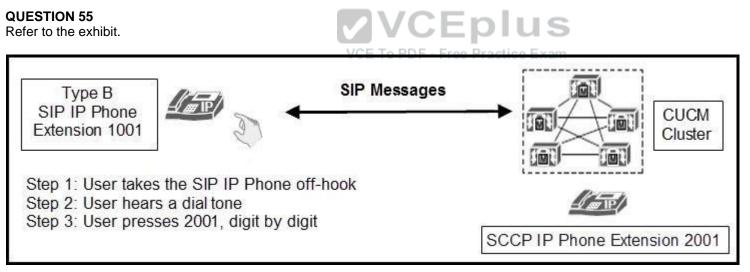
A user is going through a series of dialing steps on a SIP Type B IP phone (for example, a Cisco 7975) to call an SCCP IP phone. Both phones are registered to the same Cisco Unified Communications Manager cluster. Assuming the calling SIP phone is associated with a SIP dial rule with a pattern value of 2001, which statement about how digits are forwarded to Cisco Unified Communications Manager for further call processing is true?
