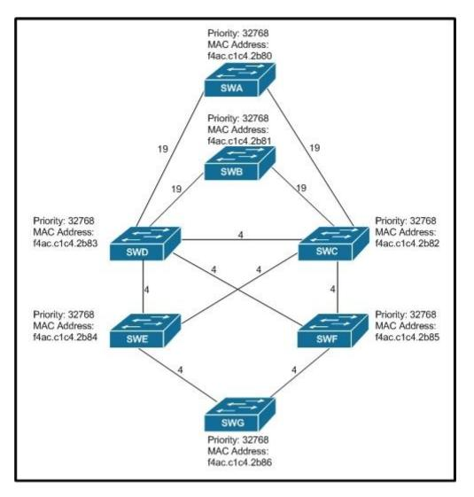
All switches have default bridge priorities, and originate BPDUs with MAC addresses as indicated. The numbers shown are STP link metrics. Which two ports are forwarding traffic after STP converges? (Choose two.)
