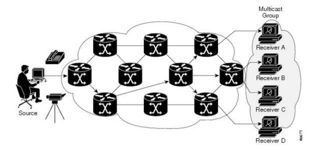
In the example shown above, the receivers (the designated multicast group) are interested in receiving the video data stream from the source. The receivers indicate their interest by sending an Internet Group Management Protocol (IGMP) host report to the routers in the network. The routers are then responsible for delivering the data from the source to the receivers.
