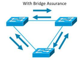
Bridge Assurance (BA) can help protect against bridging loops where a port becomes designated because it has stopped receiving BPDUs. This is similar to the function of loop guard.
