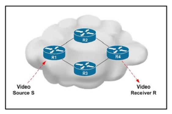
Video Source S is sending interactive video traffic to Video Receiver R. Router R1 has multiple routing table entries for destination R. Which load-balancing mechanism on R1 can cause out-of-order video traffic to be received by destination R?
