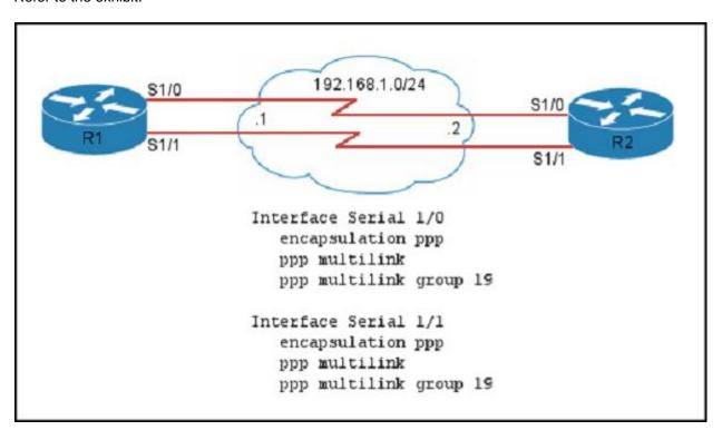
You must complete the configuration on R1 so that a maximum of three links can be used and fragmentation is supported.
