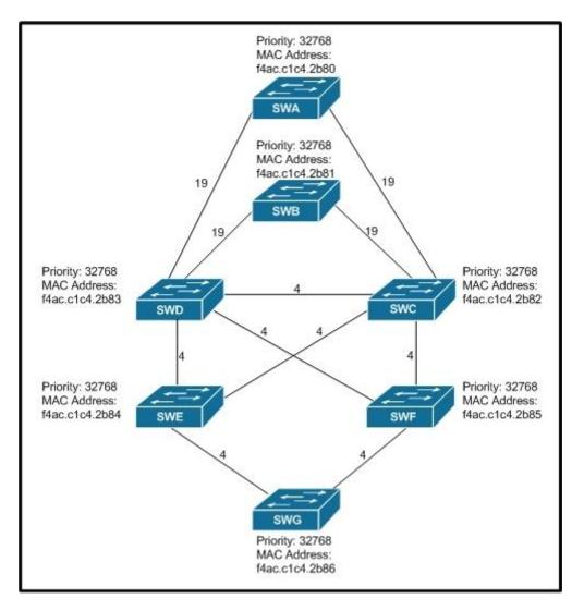
All switches have default bridge priorities, and originate BPDUs with MAC addresses as indicated. The numbers shown are STP link metrics. Which two ports are in blocking state after STP converges? (Choose two.)
