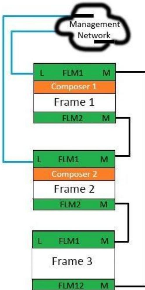
You are installing three Synergy frames for a customer PoC in the configuration shown. The composer is unable to discover the frames. What is the most likely cause of the problem?
