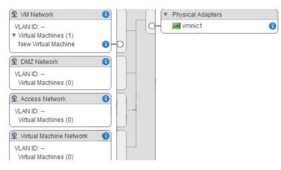
A vSphere 6.x Standard Switch is configured with 4 virtual machine portgroups, as shown in the exhibit.
