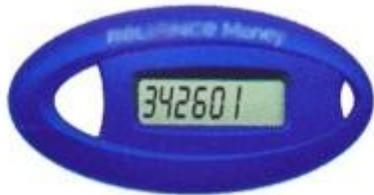
These are display-only devices that algorithmically generate security codes as part of a challenge/response authentication system. This code usually changes very quickly and is used with the PIN for authentication.
