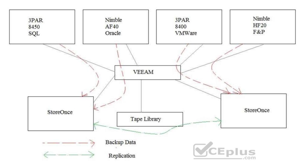
A customer has the environment shown. They currently perform application-consistent daily full backups via Veeam backup to an HPE StoreOnce device. These backups are then replicated to an alternate device using Catalyst copy. Changing business requirements have mandated the RPO and RTO for the customer's SQL databases be reduced to 15 minutes. Due to the size of the databases, it is not possible to meet this requirement with their existing backout application.
