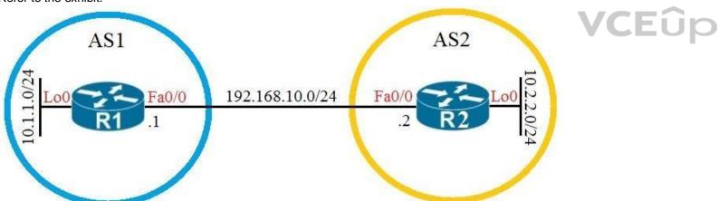
Which configuration establishes EBGP connected neighborship between these two directly connected neighbors and exchanges the loopback network of the two routers through BGP?
