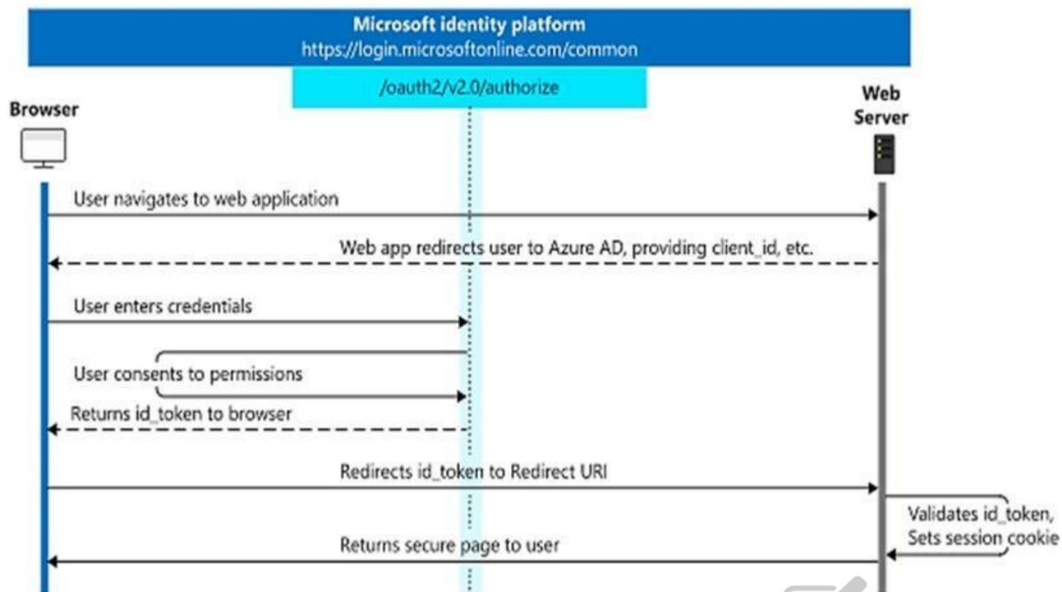
You can ensure the user's identity by validating the ID token with a public signing key that is received from the Microsoft identity platform endpoint. A session cookie is set, which can be used to identify the user on subsequent page requests.
