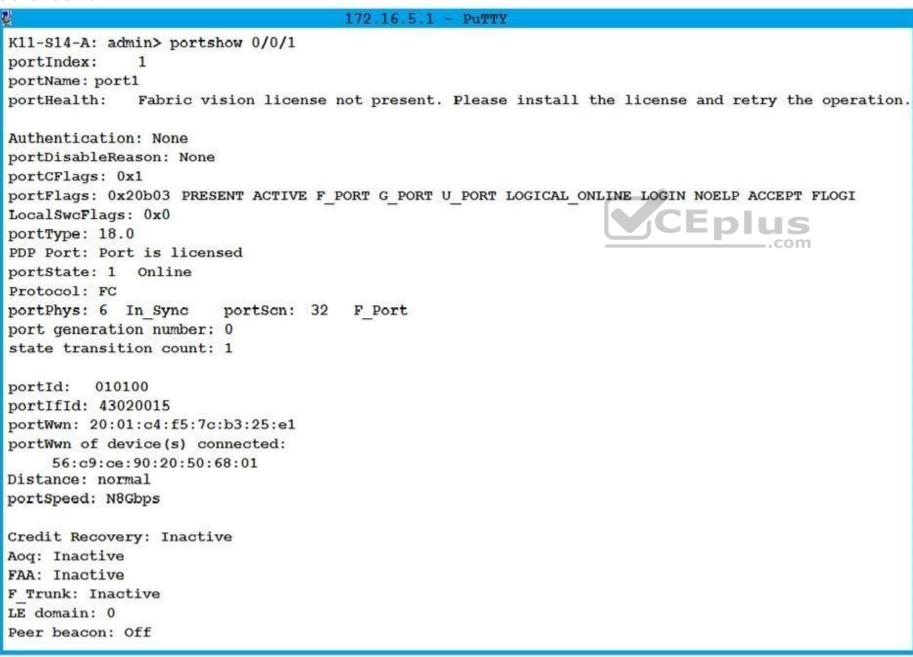
The information shown is displayed for a Nimble array you are installing. The customer's administrator has asked you for the speed at which the Nimble ports are connecting to their SAN switches, and you have run the command shown to determine the number of gigabits per second used by this port connection.
