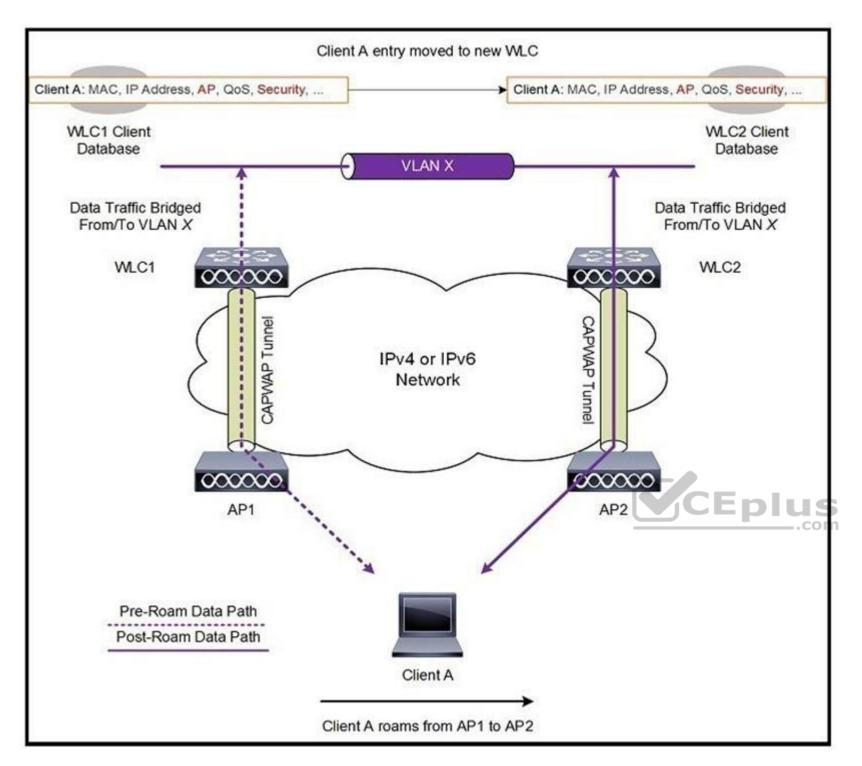
Refer to the exhibit. A client roams between two APs that are registered to two different controllers, where each controller has an interface in the client subnet. Both controllers are running AireOS. Which scenario explains the client roaming behavior?
