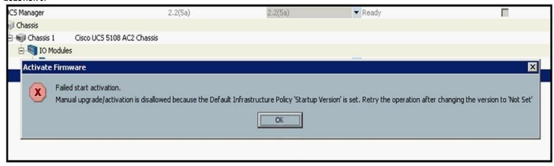
Refer to the exhibit. Cisco UCS Manager is being upgraded using the Auto Install feature, but the FSM fails. Which action resolves the issue?
