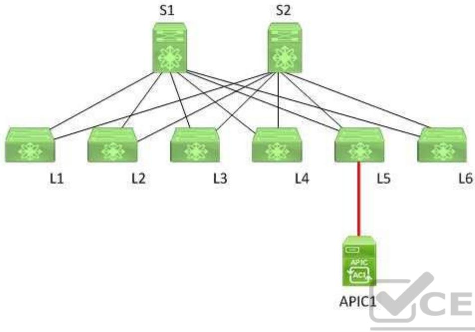
S2 has just been discovered by APIC1. Only one leaf switch has been discovered and registered with APIC1 so far. No other spine switches have been discovered. Which of the following switches will most likely be discovered next?
