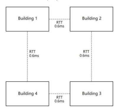
A university campus has a site topology illustrated in the exhibit. Adjacent connected buildings are connected with a single 40gb layer 3 network with a RTT of 0.6ms as depicted by each line. An architect wants to configure a fault domain in each building. CEPIUS
