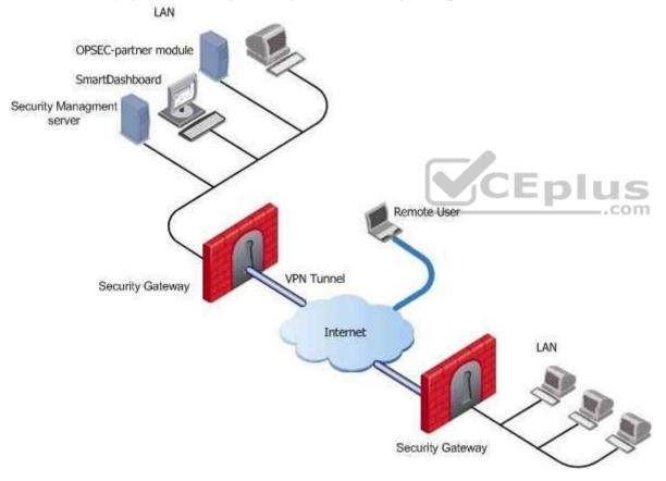
Assume an environment with gateways on different sites. Each Security Gateway connects to the Internet on one side, and to a LAN on the other. You can create a Virtual Private Network (VPN) between the two Security Gateways, to secure all communication between them.
