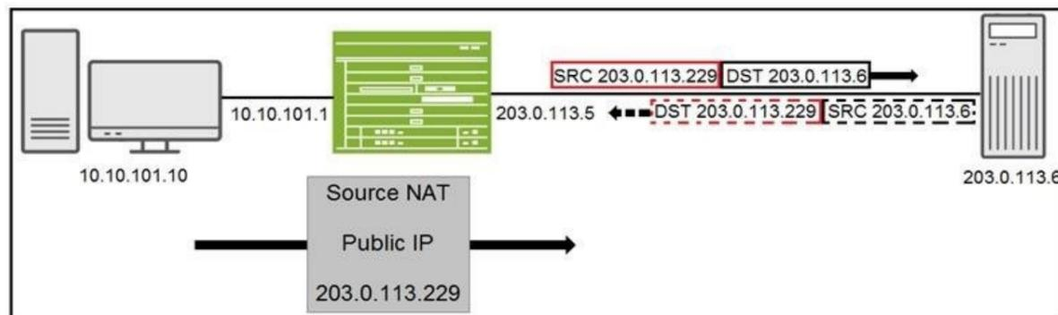
You have configured source NAT using an address pool as shown in the exhibit. Traffic is reaching the 203.0.113.6 server but return traffic is not being received by the SRX Series device.
