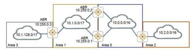
The network administrators is trying to add a remote location as area 3 to the network shown in the diagram. Based on current connection restrictions, the administrator cannot connect area 3 directly to area 0. The network is using AOS-CX switches.
